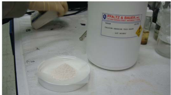
Figure A-1: Calcium peroxide to be used for Fenton oxidation of leachate
