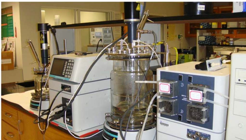
Figure A-2: Batch reactor with inline water quality measurements to be used for Fenton oxidation of leachate
