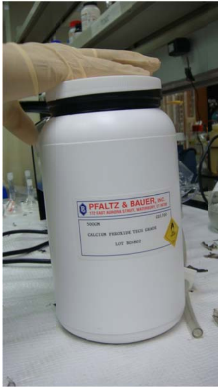
Figure A-1: Calcium peroxide to be used for Fenton oxidation of leachate
